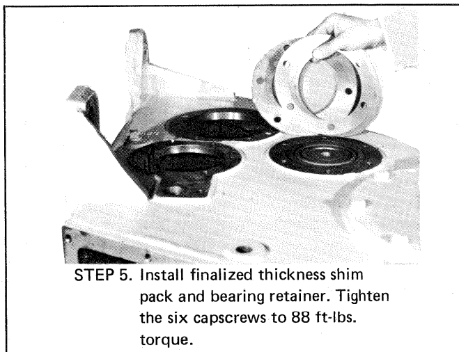
FIGURE 5-14. INSTALLATION OF INTERMEDIATE SHAFT ASSEMBLY
