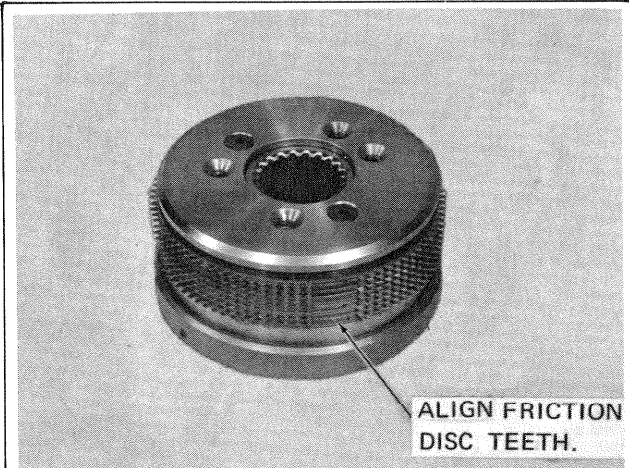
STEP 13. Align friction discs as shown.
